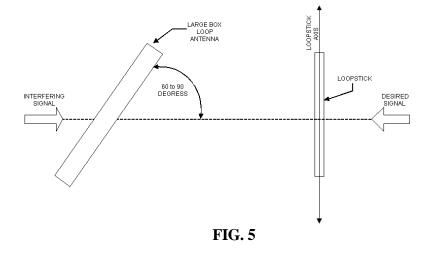
The spoiler is placed 30 to 90 cm behind the receiver antenna, again the exact amount being determined experimentally. Although the use of a loopstick is shown (the assumption being that a portable AM BCB radio is being used for reception), a box loop can also be used for the receiver. Indeed, when a communications receiver is used, both loops will be box loops.
